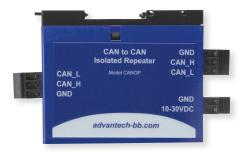
Model BB-CANOP increases the node capacity of CAN (Control Area Network) systems while protecting CAN networks from component destroying surges and transients. The BB-CANOP provides 2,000 VDC of optical isolation to separate and protect critical segments of the system from the rest of the CAN Network. It is protocol independent, allowing it to work with different CAN protocols and frame lengths.
